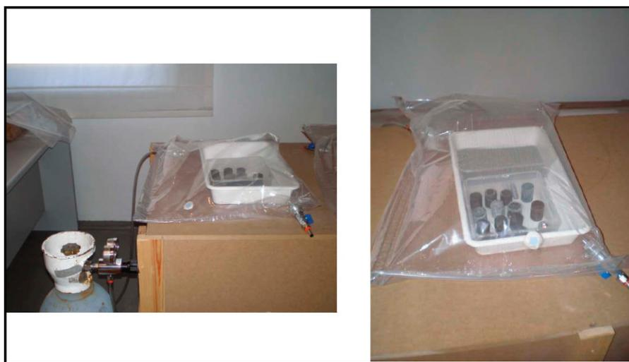
**Fig. 1.** General view of carbonation test.
