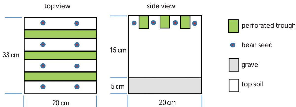
Fig. 2. Schematic diagram of the pots for the outdoor experiment with MAs on the surface of the top soil.
