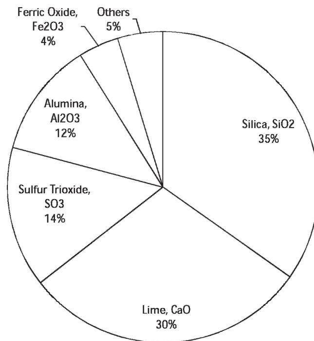
**Fig. 1.** Metal oxide composition of the MAs (% wt).
