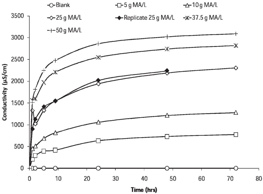
Fig. 4. Trend of conductivity development by the MAs in deionized water. The same MAs with a particle size of 2.36 to 9.53 mm that used for the plant experiments were tested.
