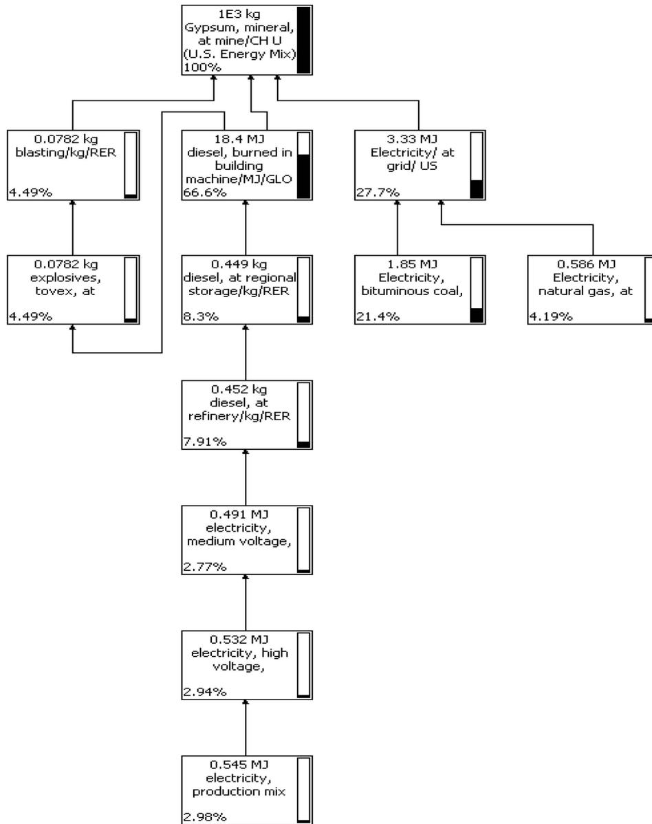
Fig. 2. SimaPro network diagram for mining virgin gypsum.
