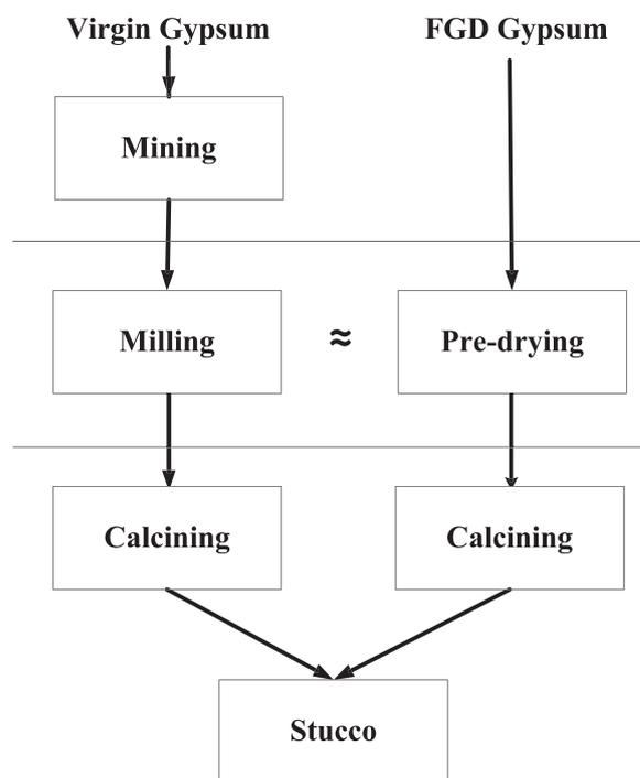
**Fig. 1.** System boundary for stucco production during wallboard manufacturing using virgin gypsum or flue gas desulfurization (FGD) gypsum.
