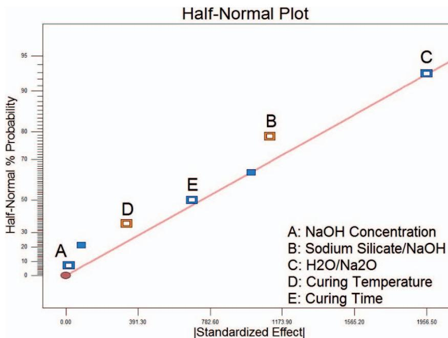
Fig. 2. Critical parameters affecting the compressive strength of geopolymer concrete.
