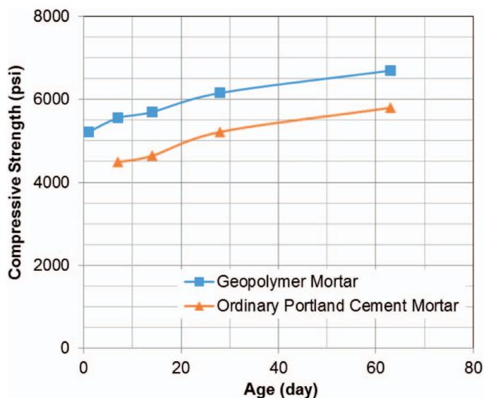
Fig. 3. Comparing the geopolymer and ordinary Portland cement mortar samples.
