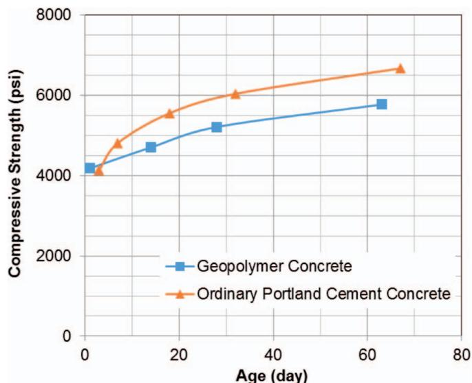
Fig. 4. Comparing the geopolymer and ordinary Portland cement concrete samples.
