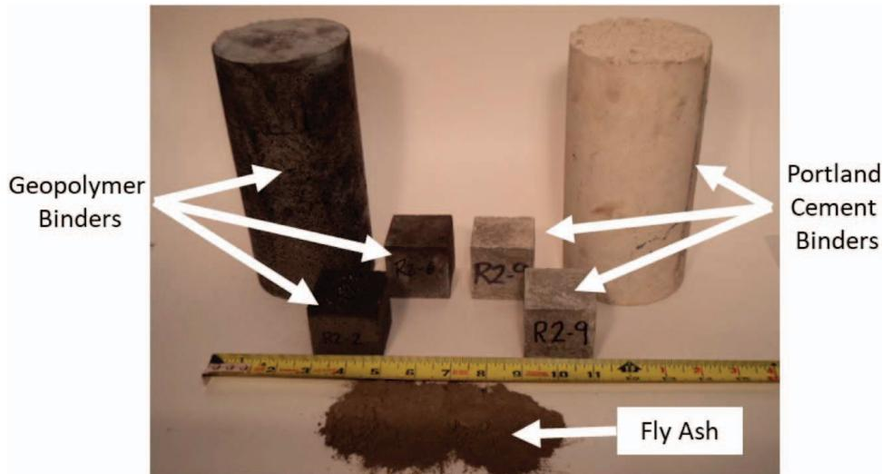
Fig. 1. Geopolymer binders made from the Carolinas fly ash vs. ordinary Portland cement binders.
